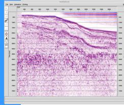
The seismic section along the MT profile (White et al. 1999, Tarits et al. 2009) (left) identifies the top of the basalt layer while the MT model (right) provides the complementary information about the bottom of the basalt layer and the structures below. MT inversion includes bathymetry (from 250 to 1400 m) and models both MT tensor and tipper.
