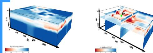
Resistivity model of the Northern part of the Isle of Skye. The model (left) shows the succession of resistive basalt cover (top), conductive Mesozoic sediments and resistive Precambrian Torridonian sandstone (bottom). The model slices (right) show the well resolved structures in the sedimentary sequence.
