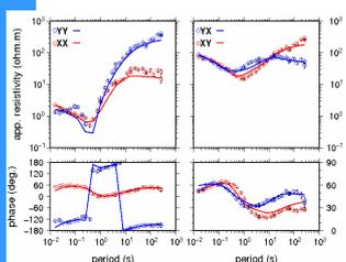
Left: Amplitude and phase of the MT impedance tensor. The amplitude is scaled into apparent resistivity. The solid line is the impedance predicted by the best fitting 3-D model. The symbols are for the observed data. XX and YY stands for the diagonal tensor coefficients and XY and YX stands for the off-diagonal coefficients.
